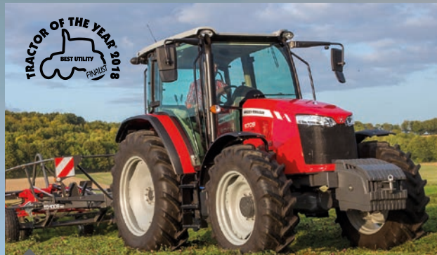
Dyna-4 transmissions now available on the MF 5708 and MF 5709 provide four change-on-the move Dynashift speeds in each gear
